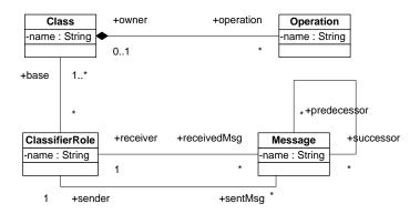
Fig. 1. A small excerpt of the UML metamodel
