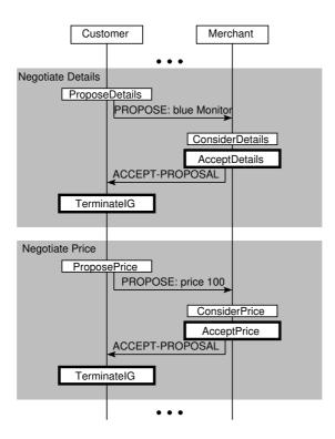
Fig. 5. (Partial) Action Message Diagram
